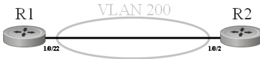
Figure 17-239. Diagram of a Routed VLAN
